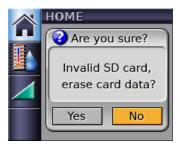
If you press "Yes", all data on the SD card will be erased. A message saying "Erasing SD card data" is displayed. Any summary data currently on the device is copied to the SD card after it has been erased. No detailed data will be saved.
