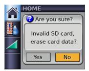
If you press "Yes", all data on the SD card will be erased. A message "Erasing SD card data" is displayed. Any summary data currently on the flow generator will then be copied to the SD card after it has been erased. There will be no detailed data.
