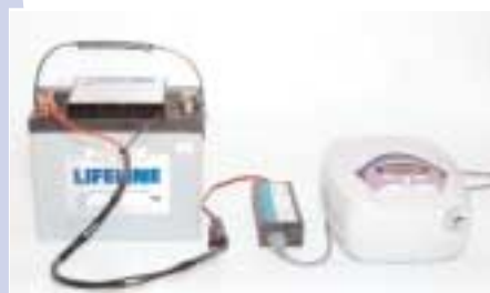
Battery setup with inverter and flow generator
